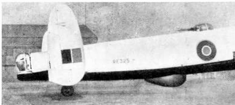
The blister enclosing the H2S scanner on the latest R.A.F. heavy bomber, the Lincoln, can be seen below the roundel.
