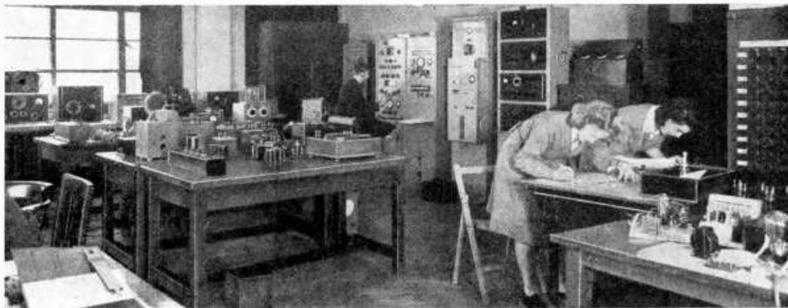
General view of the A.I.D. Electrical Standards Laboratory showing in the background (left) the standard frequency RF generator, with a beat frequency AF oscillator and harmonic analyser on its right.
